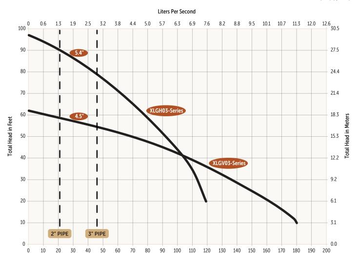
Pumps must operate within the proper range shown on the performance chart. It is the responsibility of the end user to ensure this requirement is met. Pumps operating outside the recommended range are prone to damage, excessive vibration, cavitation, poor efficiency, and may exceed nameplate amperage.
